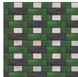
2. Middle section pattern and tones English bond Green glazed brick Black textured brick White textured brick
