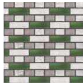
3. Top section pattern and tones English bond Green glazed brick White textured brick Light grey textured brick
